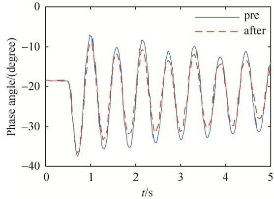
Fig. 3 Comparison of voltage phase angle of node 13 before and after partitioning
