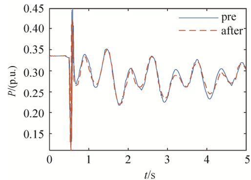
Fig. 4 Power comparison between nodes 14~15 before and after partitioning
