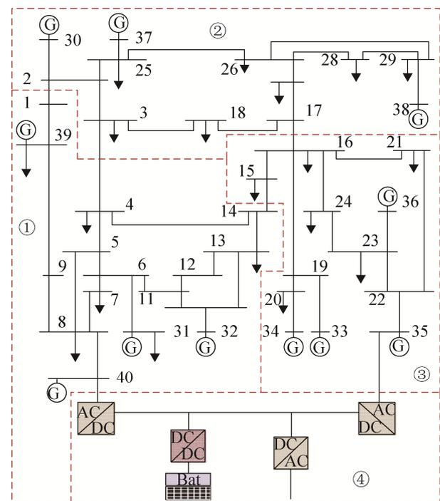
Fig. 1 IEEE 39-node 10 machine improved AC/DC hybrid simulation system
