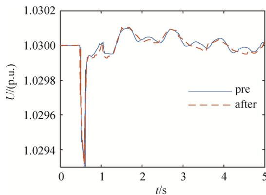
Fig. 2 Comparison of voltage amplitude of node 13 before and after partitioning
