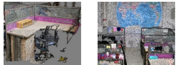
图 12 处理后点云 Fig. 12 Point cloud after processing
