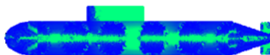
图 11 90^\circ 入射散射强度分布 Fig. 11 Scattering intensity distribution in vertical incidence
