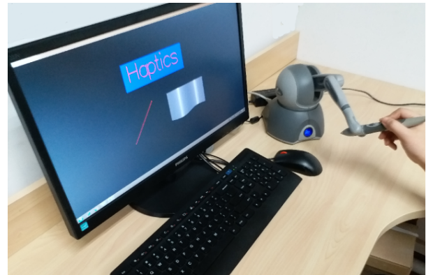
Fig. 3 3D interactive presentation system based on haptics
