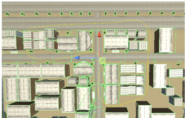
图 8 本文算法优化后的城市场景中碰撞器添加情况 Fig. 8 Collider addition in the urban scene optimized by the algorithm
