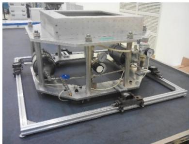
图3 实例平面气浮系统的测量现场图 Fig. 3 in-situ measurement photo of a specified planar air-bearing system
