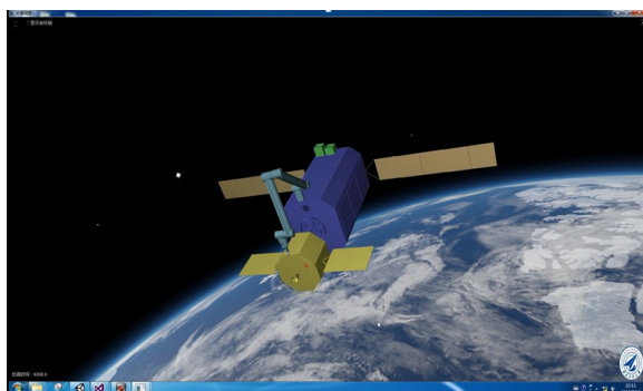
图 17 6 049 s 主星机械臂抓住目标星挂环 Fig. 17 The robot on main Sat seizes the ring on the target Sat at 6049s
