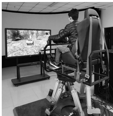
图14 林木联合采育机虚拟训练系统 Fig. 14 Forestry felling & cultivation machine virtual driving training system
