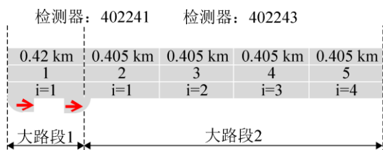
图5 I-80E 大路段1和大路段2METANET 建模示意图 Fig. 5 Road section 1 and 2 in METANET of I-80E highway
