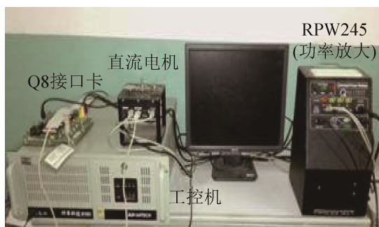
图4 直流调速系统硬件连接 Fig. 4 Hardware connection of DC speed regulating system
