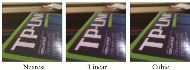
图 8 频域中不同插值方法得到的重聚焦图像 Fig.8 Refocusing images obtained by different interpolation methods in frequency domain
