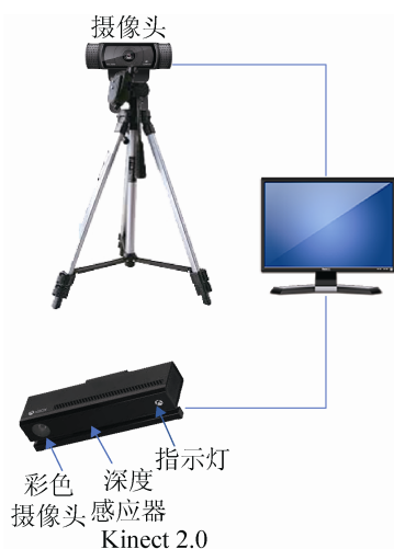
图 2 系统硬件架构 Fig. 2 Hardware structure
