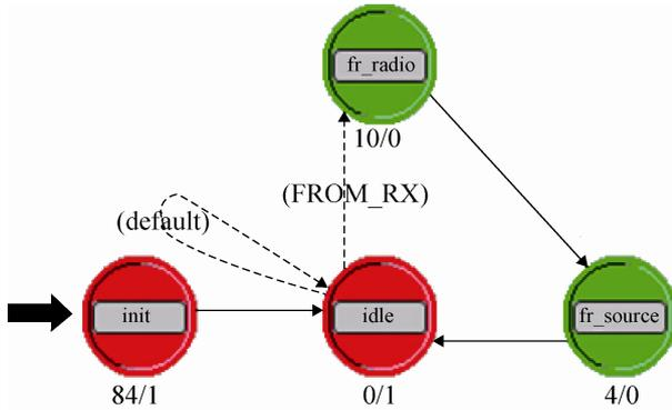
Fig. 5 TDMA protocol satellite process model
