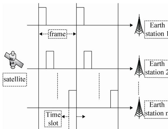
Fig. 2 TDMA satellite working principle diagram
