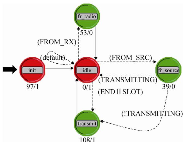
Fig. 4 TDMA protocol ground station subnet process model
