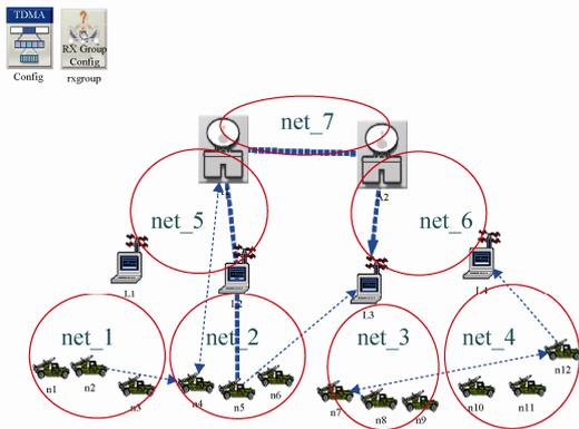
Fig. 10 Hierarchical routing selected path graph
