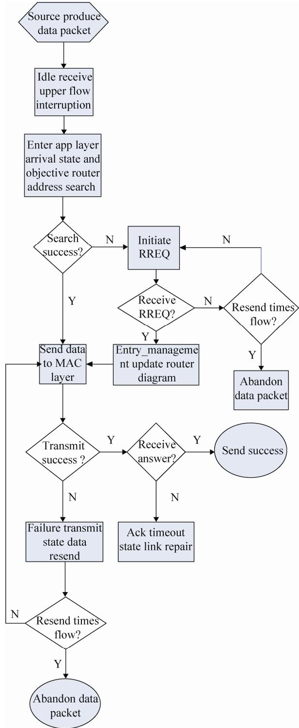
Fig. 6 send packet flow chart
