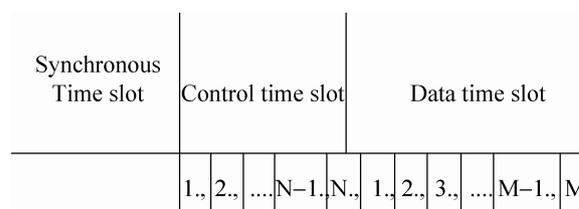
Fig. 3 frame structure
