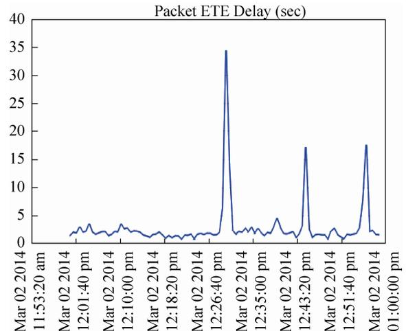
Fig. 12 Hierarchical routing protocol average end-to-end delay
