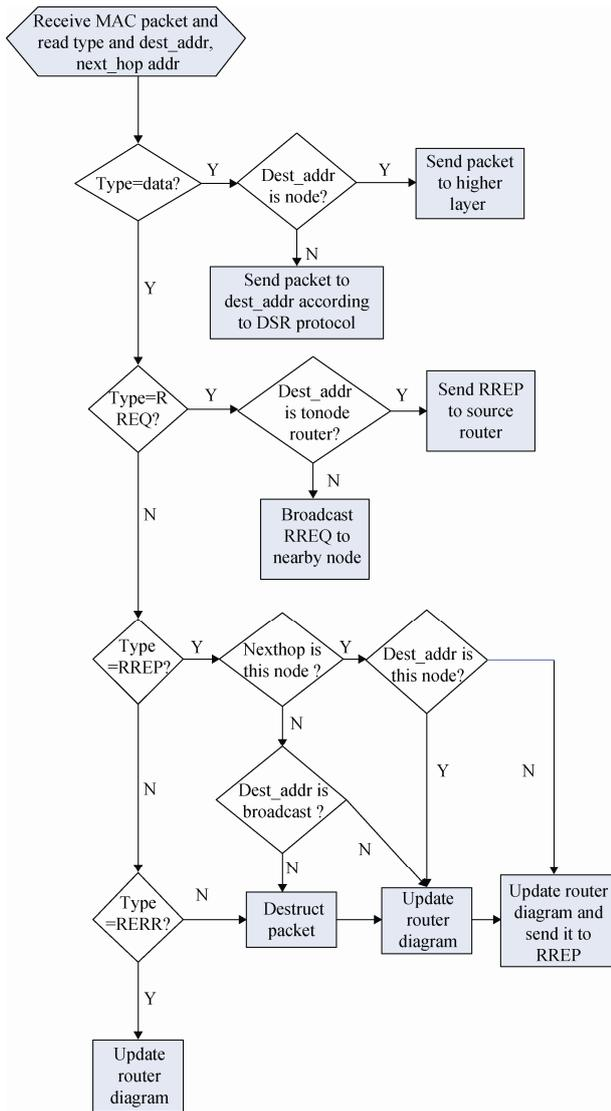
Fig. 7 The flow chart of receives packets
