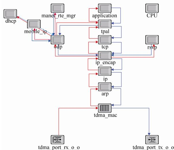
Fig. 1 Communication network protocol framework model
