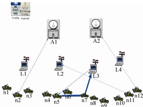
Fig. 11 The DSR routing selected path graph
