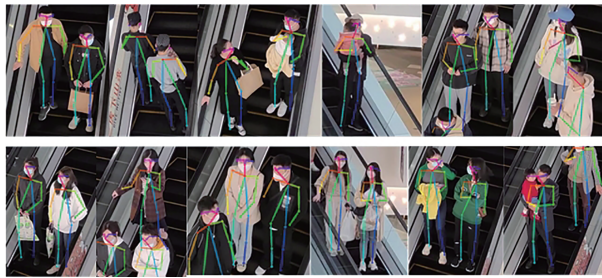
图12 遮挡重叠情况的姿态识别结果 Fig. 12 Attitude recognition results for occlusion and overlap
