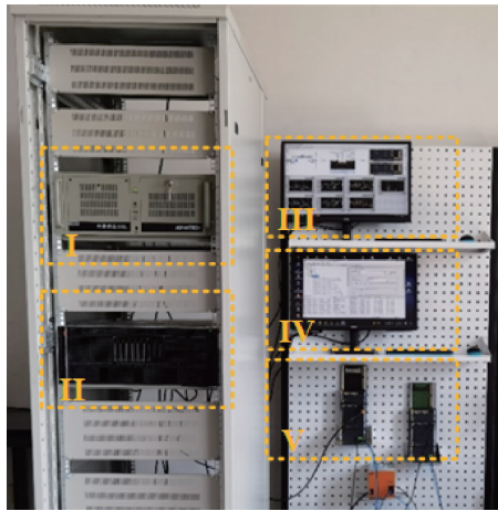
图6 大型风电机组数字孪生仿真系统 Fig. 6 Digital twin simulation system for large wind turbines
