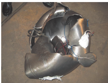
图11 耐压壳内爆 Fig. 11 Pressure hull implosion
